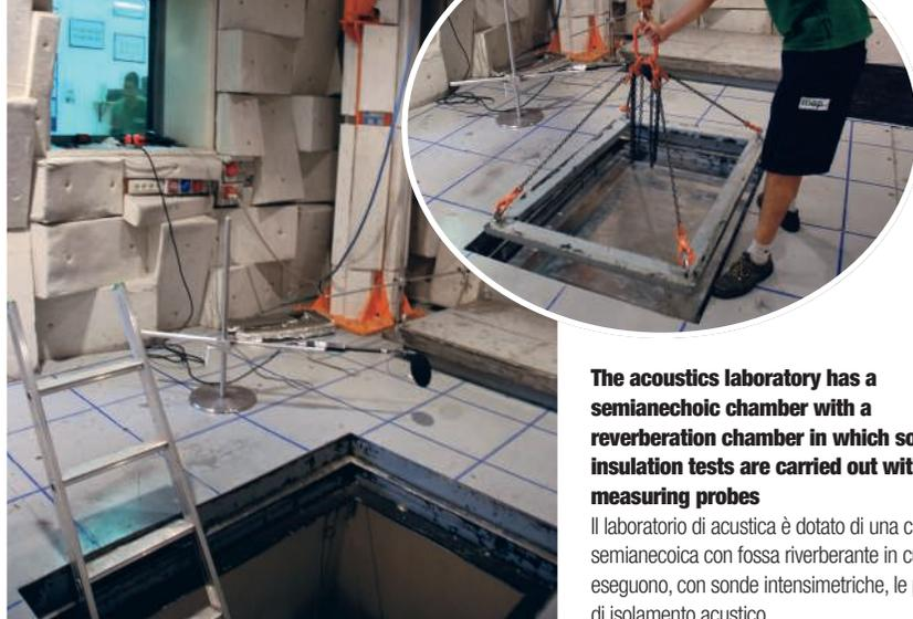
**The acoustics laboratory has a semianechoic chamber with a reverberation chamber in which sound insulation tests are carried out with measuring probes**
