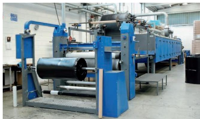
**A phase of production: coupling sound insulation and sound absorbing materials**
